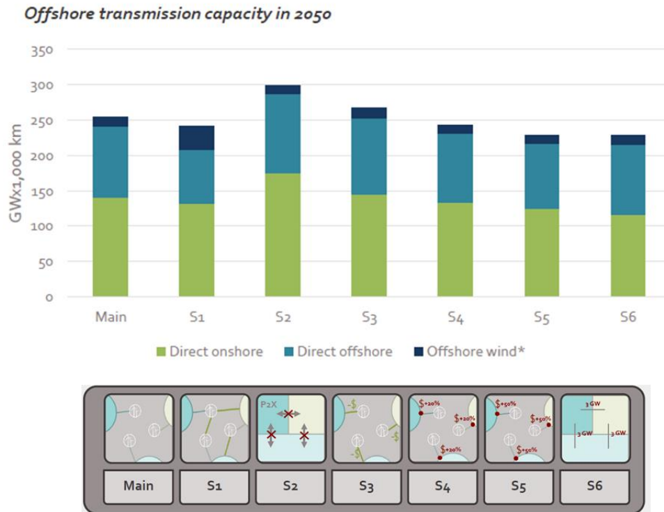
Figure 11 - Benefits in term of installed capacities of transmissions between a situation where investments in hybrid projects are possible (S1) and a reference situation where wind farms can only be connected to the nearest shore (Main), and a situation where hydrogen exchanges between zones are not possible (S2)
